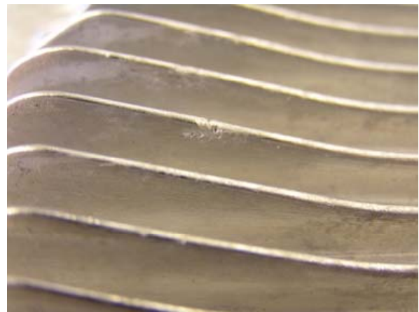
Fig. 4: Casting defects on cooling fins produced from alloy AZC1231
