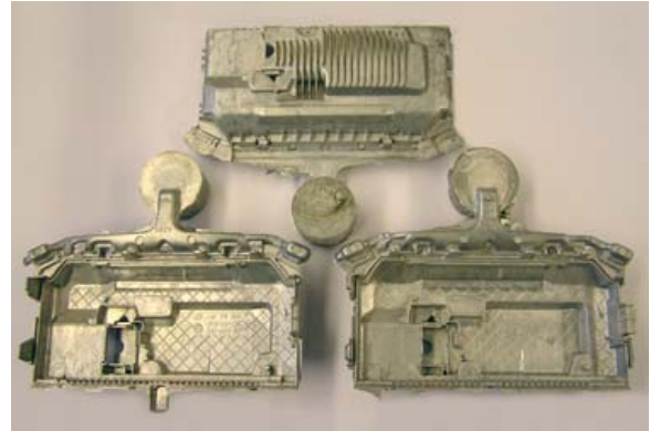
Fig. 3: Housing cast by cold chamber high pressure die casting using the newly developed secondary alloy AZC1231
