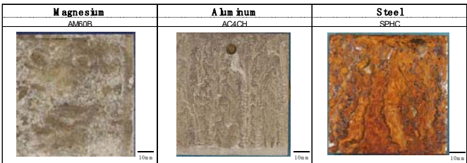
Fig.10 The photographic views of the surface after SST
