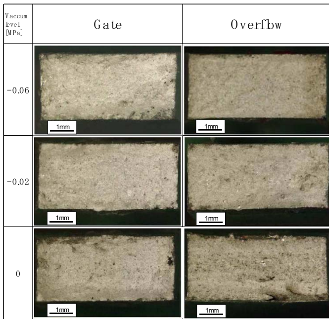
Fig.6 Photographic views of the fracture surface
